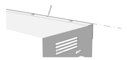
Remove the screws and top bracket from the fire. Using it as a template mark the fixing holes on the wall, drill the holes with an M10 bit and fit the rawl plugs. Using the 60mm screws fix the bracket to the wall.
