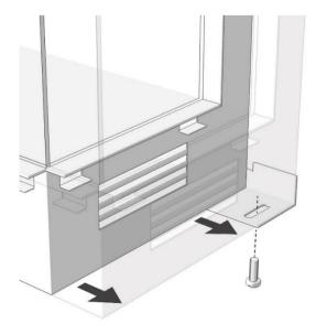
Before any further work is completed now your fire is secure, make sure the mains cable is <u>tightly</u> fitted underneath the fire.
