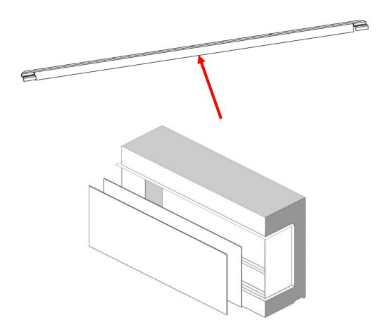
Using the foam tape provided in the accessory pack, apply across the length of the top bracket's front face to keep the projection screen secure. Now the reflective glass screen has been removed, screw the top bracket back into place and add the projection screen. Place the fuel bed back into the fire, reconnect the cable **A** underneath and replace both the screws at either side.
