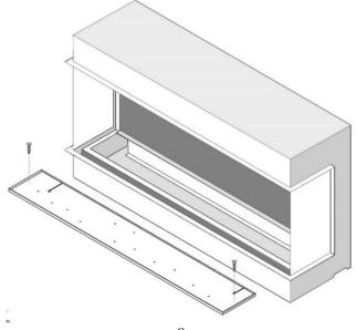
You will need to carefully remove both screens, to do this unscrew the top bracket holding them in place.
